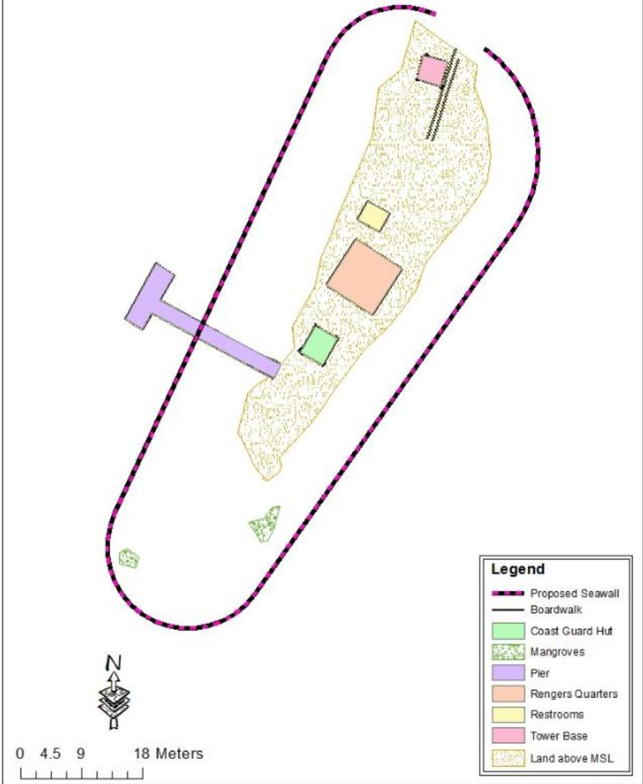
Figure 10.1A Proposed land reclamation extent for South Point rehabilitation.
