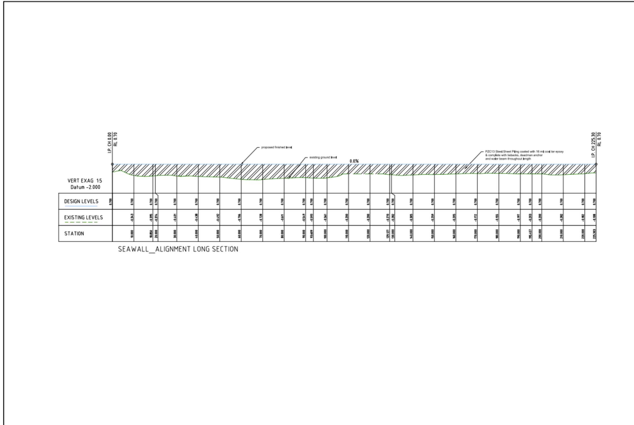
Figure 10.3.2 Twin Caye Steel Sheet Pile Seawall General Arrangement Plan (Option C)
