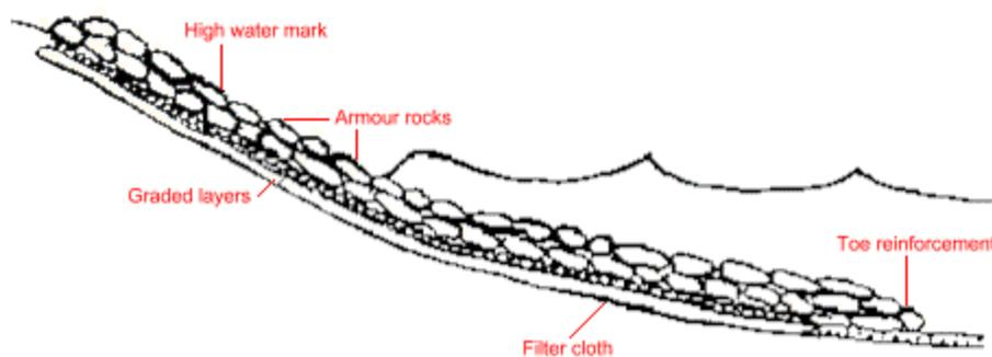
Figure 8.1.5 Schematic Rock Revetments
