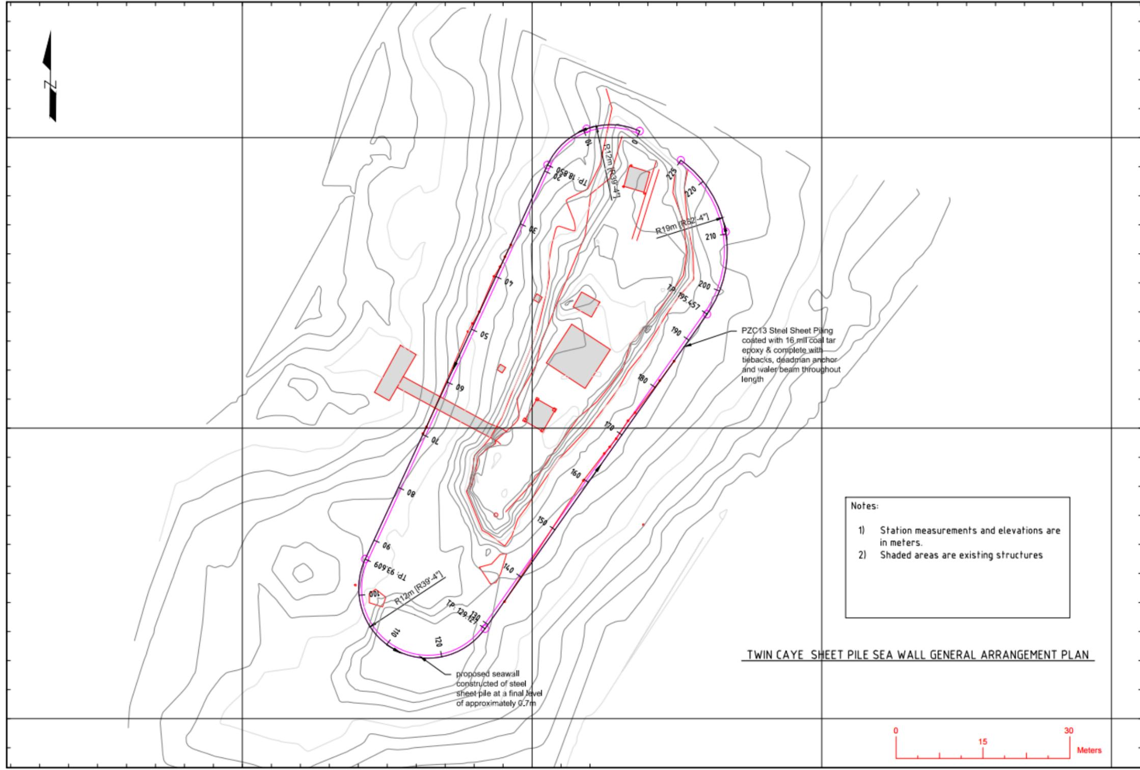
Figure 10.3.1 Twin Caye Steel Sheet Pile Seawall (Option C)
