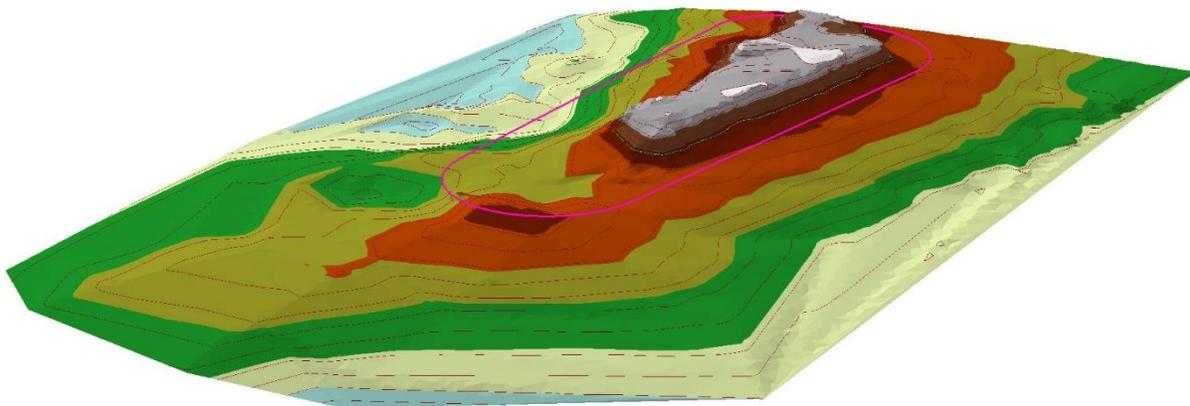
Figure 10.1 *Topo-bathymetric surface with Proposed Reclamation Extent (pink line)*
