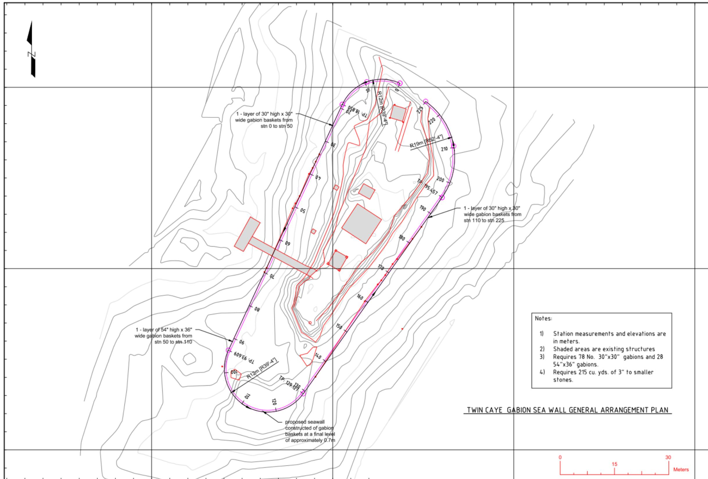
Figure 10.1.1 Twin Caye Gabion Seawall (Option A)
