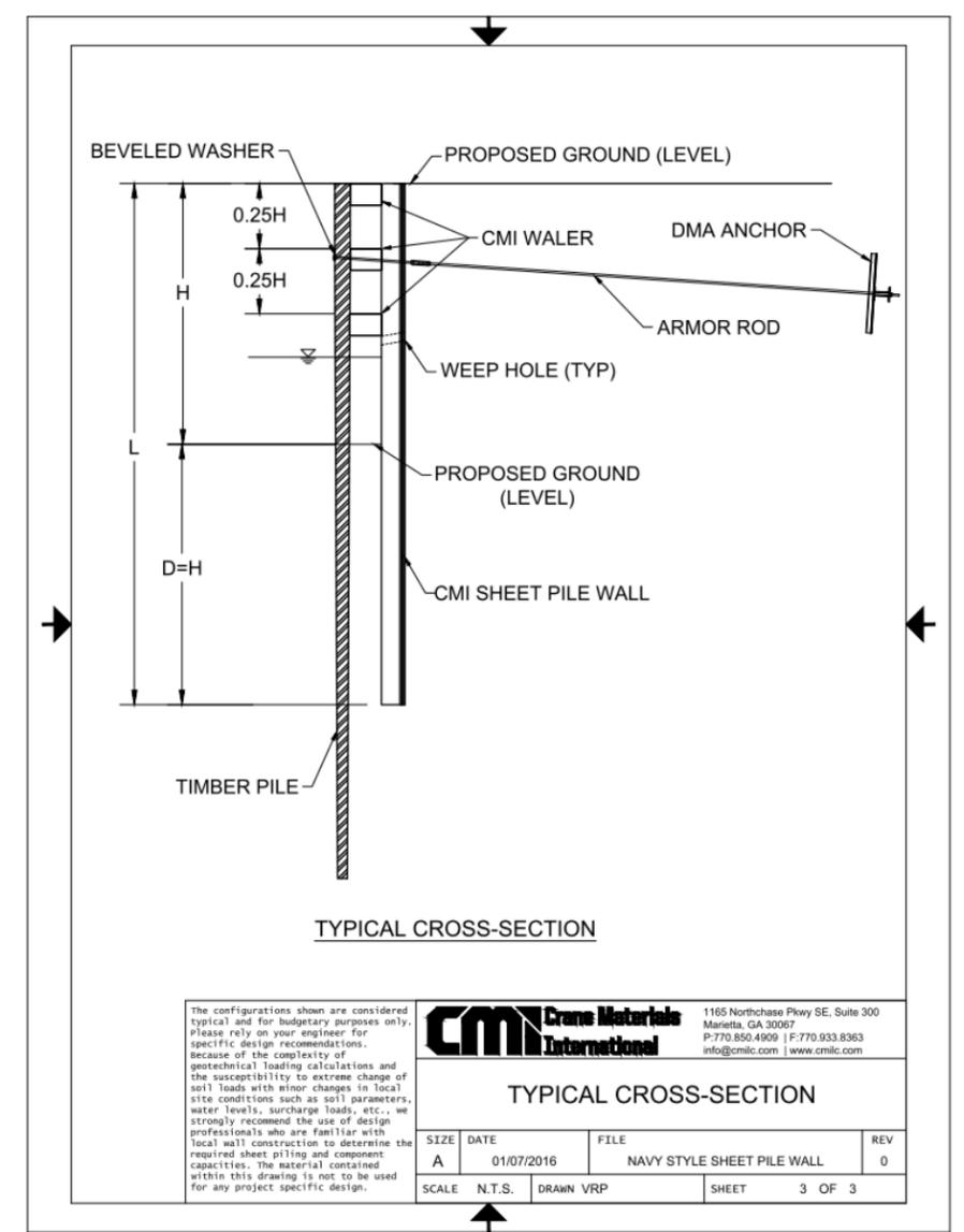
Figure 10.2.3 (a) Elevation View of the CMI Vinyl Sheet Pile Wall; (b) Plan View of the CMI Vinyl Sheet Pile Wall; (c) Typical Cross-section view of the CMI Vinyl Sheet Pile Wall
