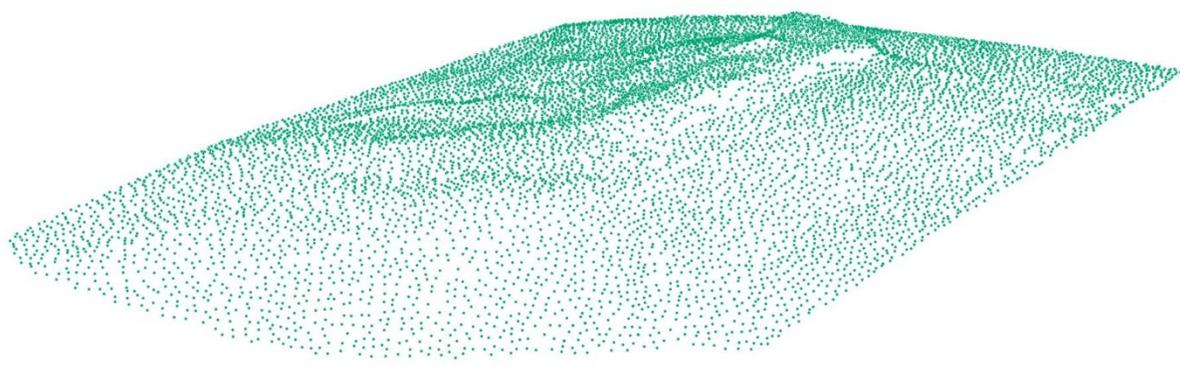
Figure 7.1.2 *Topo-bathymetric point cloud*
